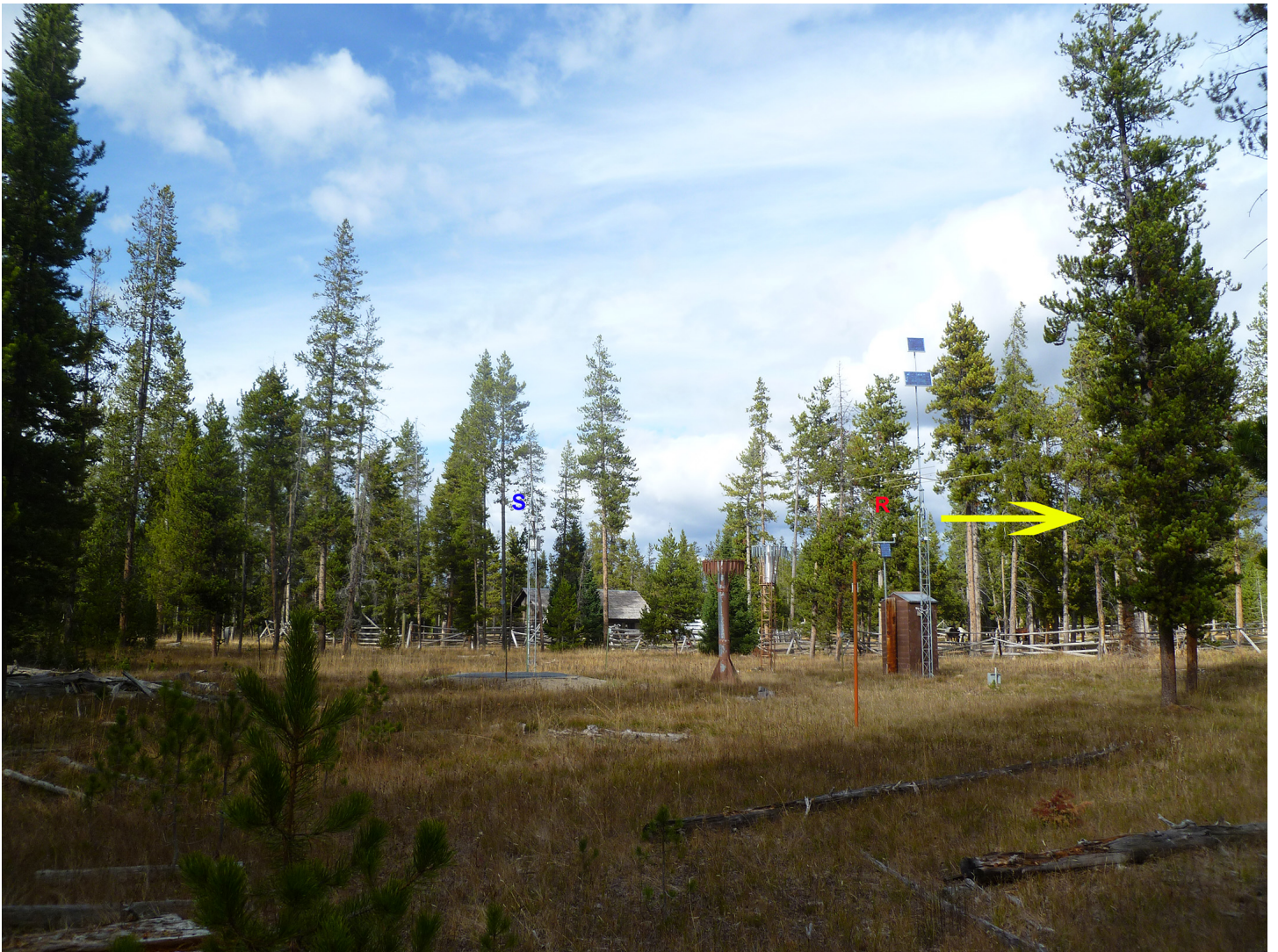
Figure 5: Photograph of the south entrance SNOTEL / RAWS installation. S = SNOTEL thermometer. R = RAWS thermometer. Yellow arrow = location of tree line to the south of the RAWS. The photographer is standing in front of the southerly tree that is closest to the SNOTEL thermometer.
